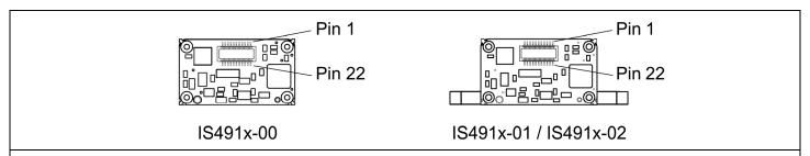
Figure 32. Imaging Engine Interface Connector
